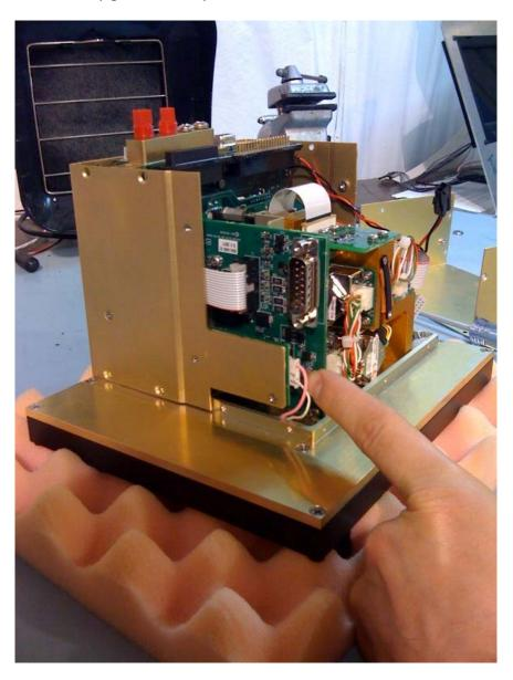
Next remove the 14 conductor cable plugged into the AHRS as shown below. When assembling, this cable's connector is marked with a triangle and should be matched up with the triangle on the AHRS connector. In the picture the red conductor is towards the screen and the cable comes back over the connector.
