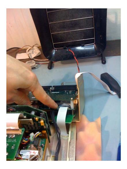
Verify it is seated firmly by applying gentle pressure across it. If you feel that you were able to press it down further, remove the silicon holding the connector to the board as it was not effective. Apply additional silicon across the top surface and on both sides of the board.
