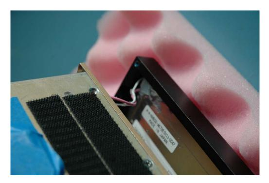
Silicon may be holding white and pink wires keeping the rear assembly from pulling away from screen. If this is the case, gently hold onto wires and pull rear assembly away from bezel 1". Gently press on the black connector on the back of the screen to verify it is fully seated.
