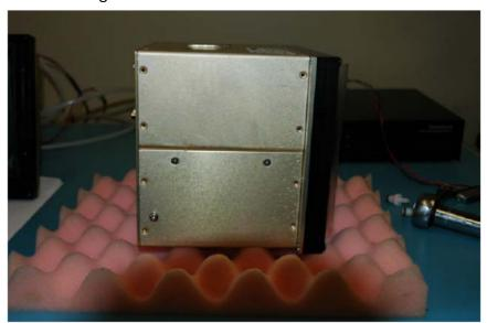
Remove all screws that hold the rear cover. 10 from the left and right side and 6 screws on the bottom and top.
