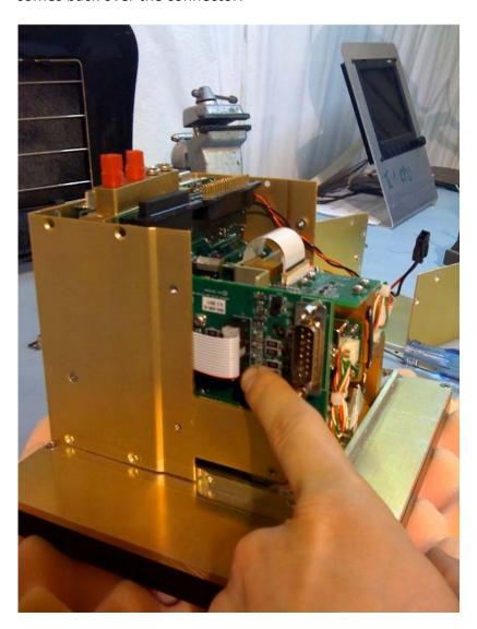
Pull straight up on the top cover assembly and lay it on the table. The LCD connector is shown in the picture below.
