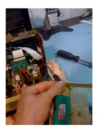
Pull straight out on the connector as shown below. When assembling, this connector is keyed and will only go in one way.
