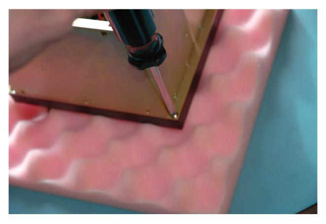
Put unit screen side down onto foam pad. Remove four corner screws as shown above. Rear case assembly will pull off screen bezel.
